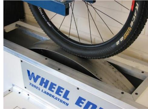
Fig. 2. Rolling Resistance testing machine at Wheel Energy.
